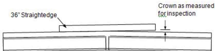
Figure 112B Crown Inspection – Side View
