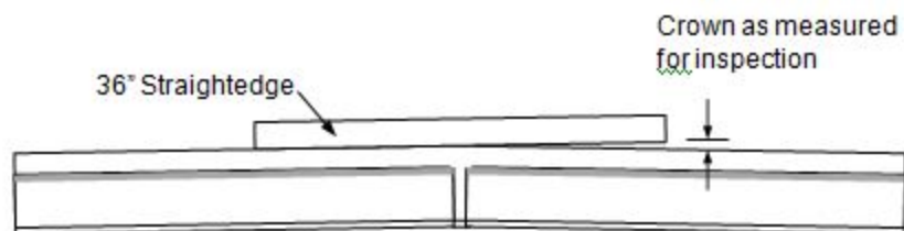
Figure 110L Crown Inspection - Side View
